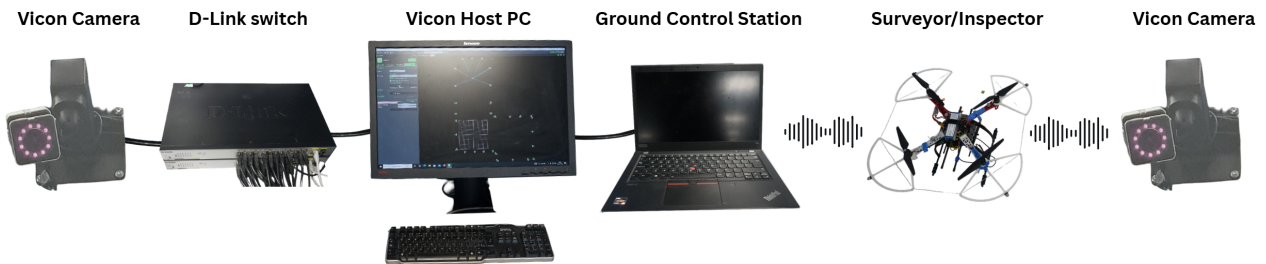
Figure 2: A high level flow diagram on the communication for localisation.
